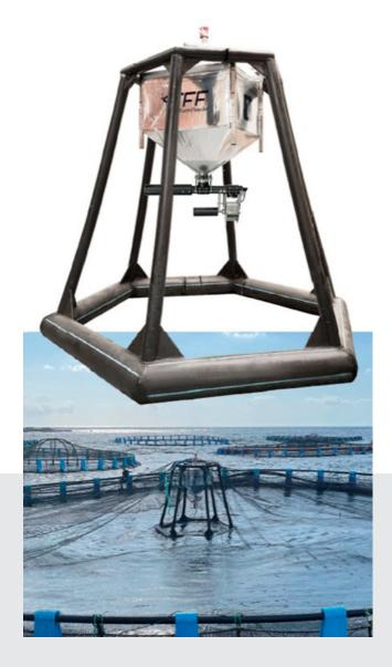
Function and Application: The solution allows automated and autonomous feeding of a fish cage in the sea. By means of algorithmic systems, it is able to control each dose and the necessary dosing time on a daily basis. It has a specific API that facilitates its integration with other systems and is enabled to collect information from external sensors for feedback and improved.
